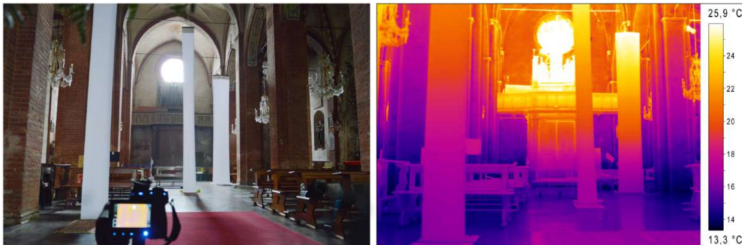
Fig. 4 Central nave: Infrared microclimate analysis. Scan at 1h45' after the start of heating (April 14 th , 2021).
