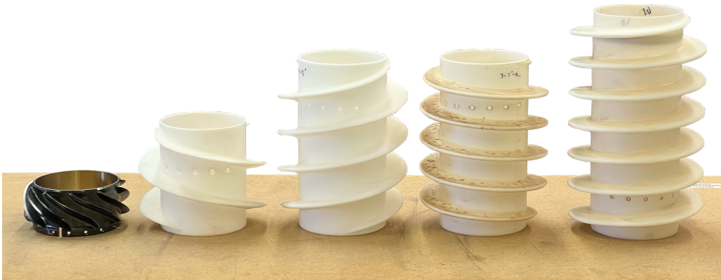
Fig. 2.3 Screw prototypes for the EELS robot active skin propulsion
