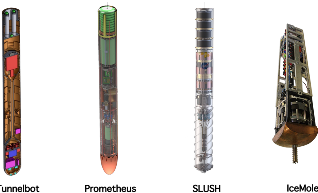
Fig. 1.4 Examples of Cryobot designs, including Prometheus [2], Tunnelbot [3], SLUSH [4] and EnEx IceMole [5]
