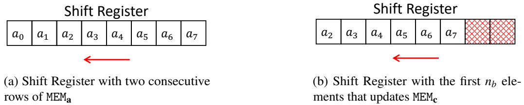
Fig. 5.3 Shift Register content to rotate MEM_a by b_2
