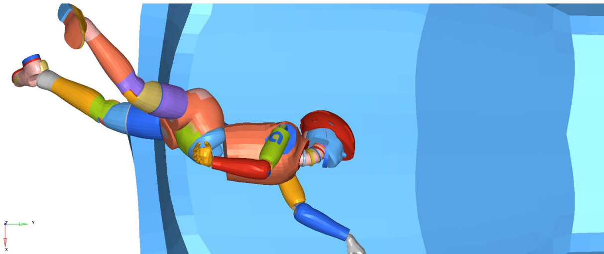
Fig. 13. Instant of the impact of the head with the hood (130 ms after the impact).
