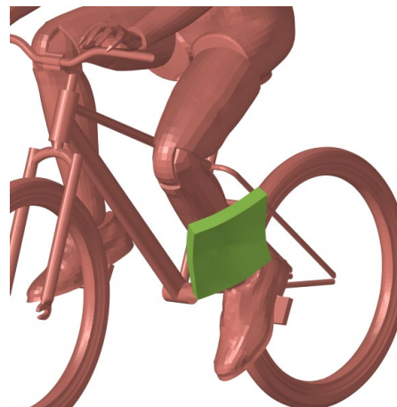
Fig. 8. Position of the foam during the impact phase.
