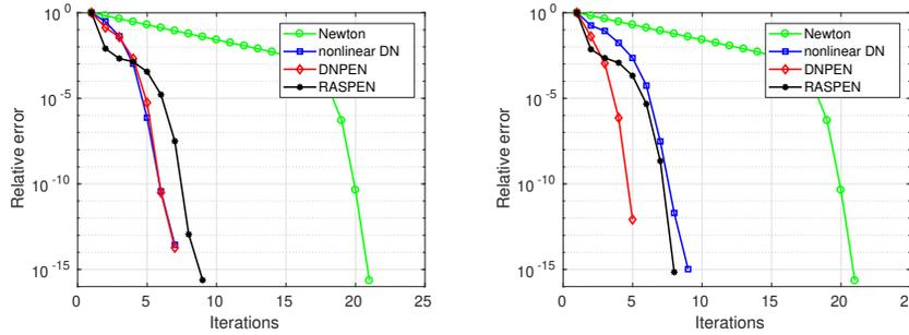
**Fig. 4:** Comparison of DNPEN (with optimal  $\theta$ ) with unpreconditioned Newton, nonlinear DN (with optimal  $\theta$ ) and RASPEN for a symmetric partition (left) and an asymmetric partition (right).
