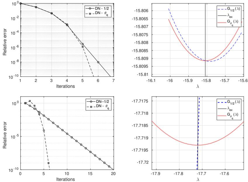
**Fig. 2:** In the left panels, we show the convergence curves, and in the right panels we plot  $G_\theta(\lambda)$ . The top-row refers to a symmetric decomposition, and the bottom-row to an asymmetric one.
