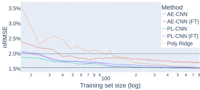
Fig. 3. Learning curves for different models. The upper dotted horizontal line is 2% of nRMSE. The lower horizontal line is 1.54% nRMSE, the final error obtained by the Polynomial Ridge. The x -axis is the number of training samples (log scale) while the y -axis is the nRMSE computed on the test set. Deep Feature extractors are able to obtain lower prediction error with a smaller training set.
