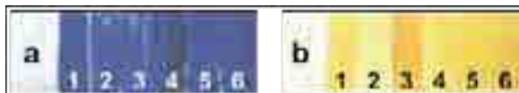
Figure 1. Retouching paints: Leningrad (1), Schmincke (2) RestaurArte (3) Rembrandt (4), Gamblin (5) and Kremer (6) with ultramarine (a) and cadmium yellow (b) pigments.
