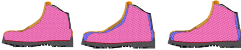
Fig. 3.7 Different configuration of the system (MODEL A on the left, MODEL B in the middle, and MODEL C the right one), the blue part represents the air gap, the pink one the feet.
