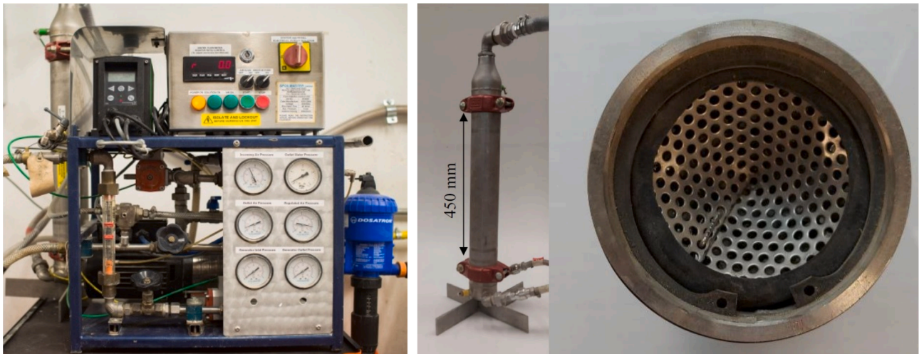
Fig. 3. Left: Laboratory scale foam generator at TUSC laboratory (Martinelli, 2016); Right: Generation cylinder (Peila et al., 2008).
