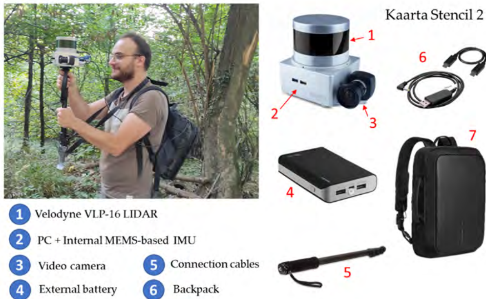
Figure 7. Kaarta Stencil 2–16 wearable mobile mapping system used: main components and a photo taken during the data acquisition.
