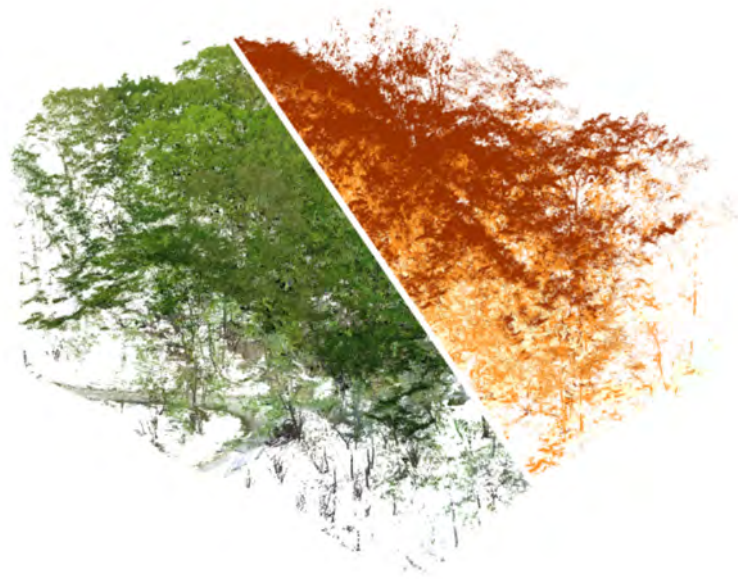
Figure 11. Point cloud acquired by the DJI L1 sensor, visualized in RGB (left) and in return number classification (right).
