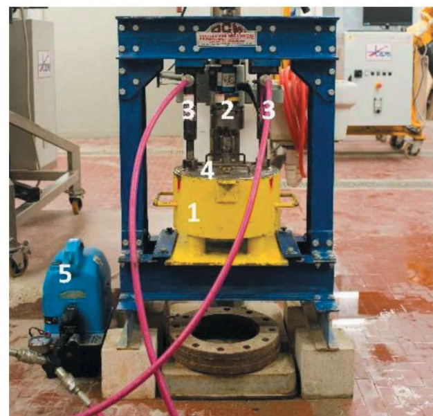
Figure 13. Schematic diagram and picture of the dynamic adhesion test apparatus. 1. steel container; 2. torque transducer; 3. hydraulic pistons; 4. steel cover; 5. hydraulic unit.
