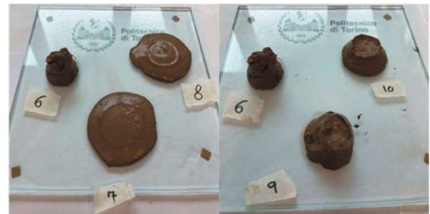
Figure 5. Mini Flow tests for “Reggio” clay. IDs are labelled.
