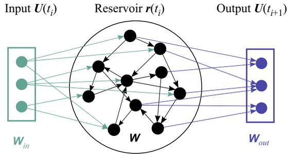
Figure 3. Schematic representation of an echo state network.
