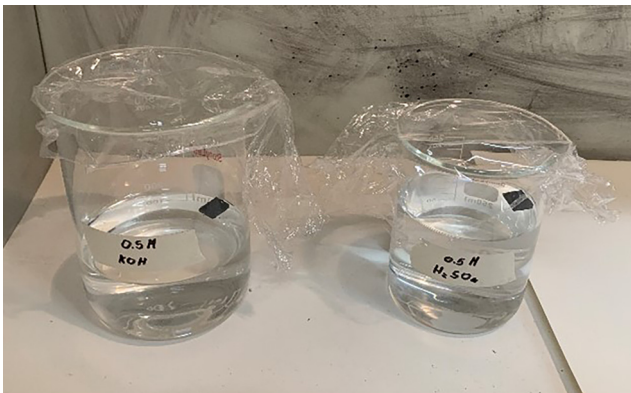
Figure 11 Experimental setup for the corrosive tests
