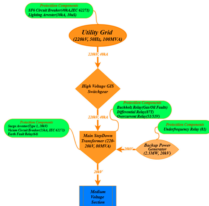
Figure 6. HV section of the power distribution network.
