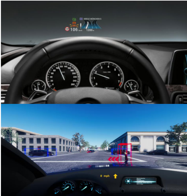
Fig. 4: Top : small HUD displaying small images and text on the bottom of the windshield. Bottom : full windshield HUD displaying a bounding box matching the position of a pedestrian crossing the road. Images adapted from BMW website and [35], respectively.
