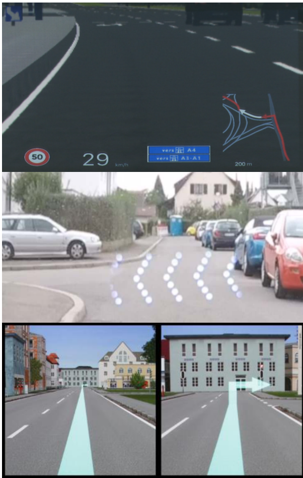
Fig. 10: Top : map pathway, displaying a map where the route to follow is highlighted [92]. Center : turning instructions, set of chevrons pointing to the turning direction [90]. Bottom : virtual carpet, a continuous path indicating the direction to follow [72]. Images adapted from the respective studies.
