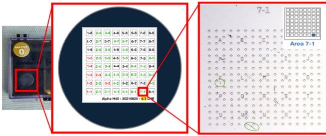
Figure 2. (left) Photography of one of the three samples used for the study. (center) Schematic view of the different numbered zone on a substrate. (right) Optical microscope view of a numbered zones (here zone 7-1) on a marked silicon substrate (9 mm × 9 mm) where are deposited nanowires. Distance between two crosses is 15 µm.
