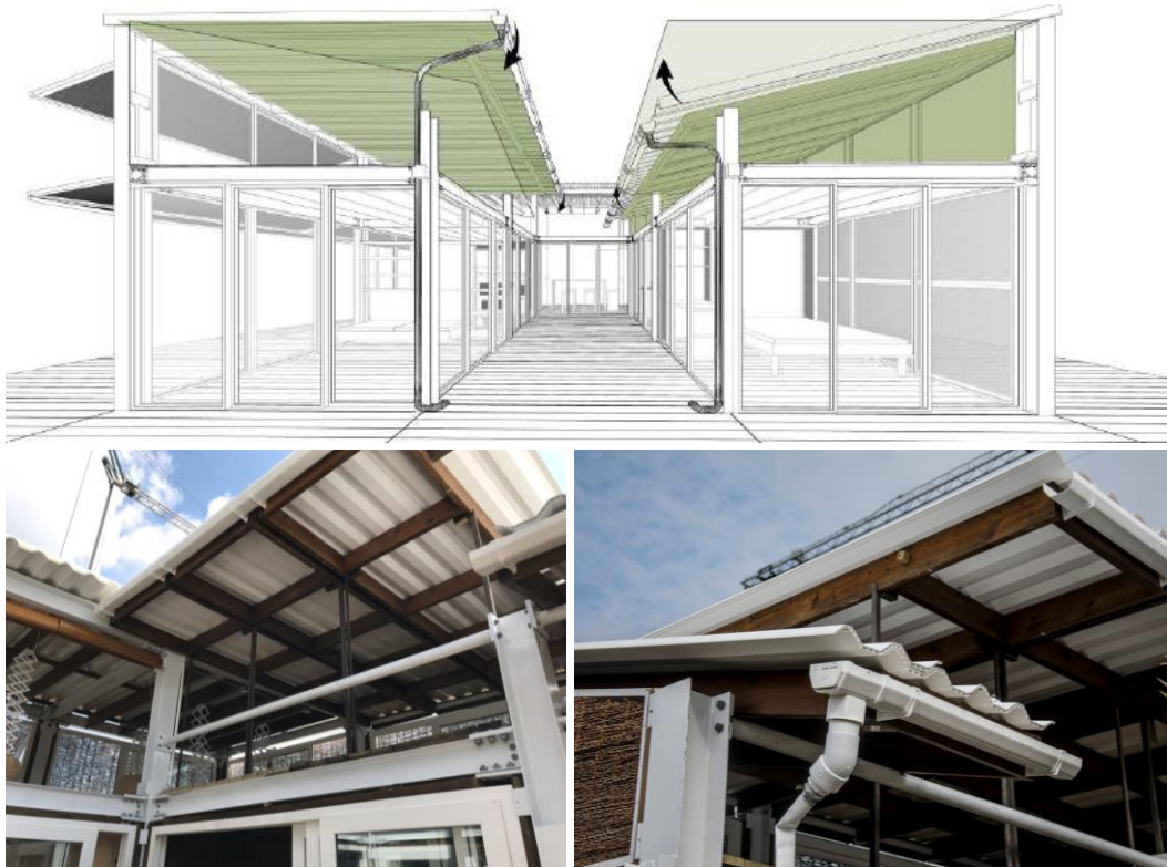
Figure 122. The movable roof: Possibility of increasing the volume of the dwelling by ceiling movement.
