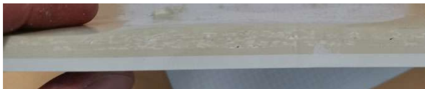
Fig. 5 Cross section of shower tray with rGFRP
