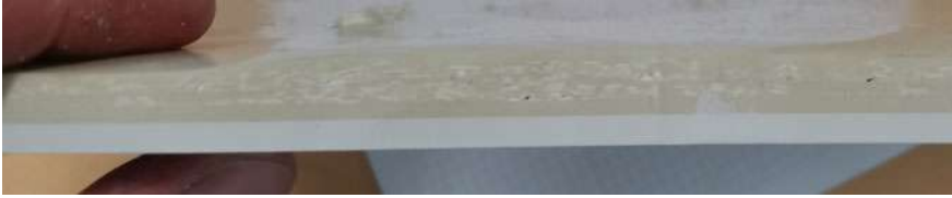
Fig. 5 Cross section of shower tray with rGFRP
