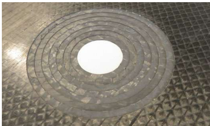
Fig. 2 Removed defect caused by an impact
