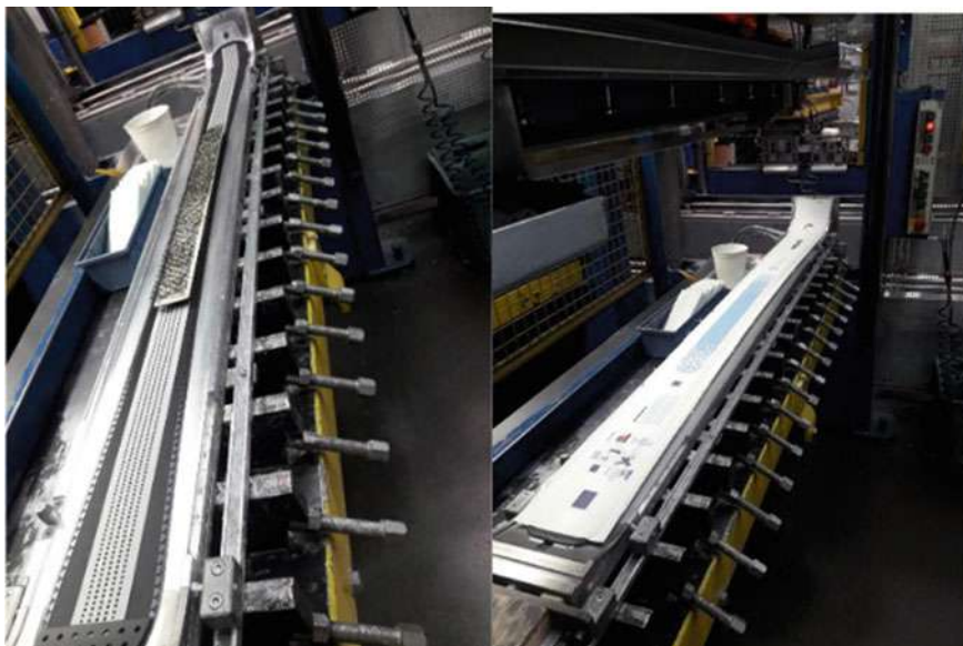
Fig. 11 Manufacturing of a demonstrator ski with the reinforcement part made from recycled material is located in the center area
