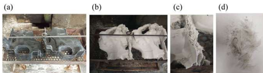
Fig. 6 a Waste Ref. B in Solvo Line oven tray, b Obtained product, c and d Long rGF with high filler content
