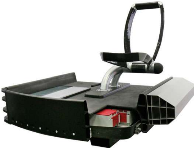
Fig. 1 Demonstrator of use-case 3—reusable structures for vehicles
