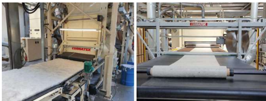
Fig. 17 Cormatex industrial production of rGF mat
