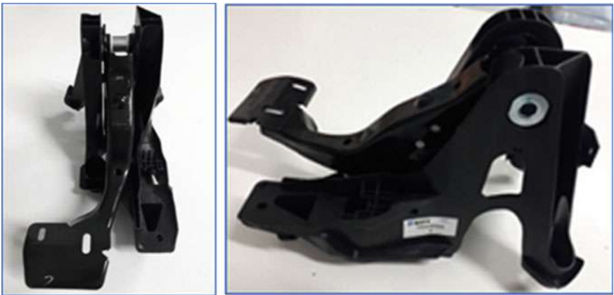
Fig. 7 Pedal bracket prototype ready for validation test
