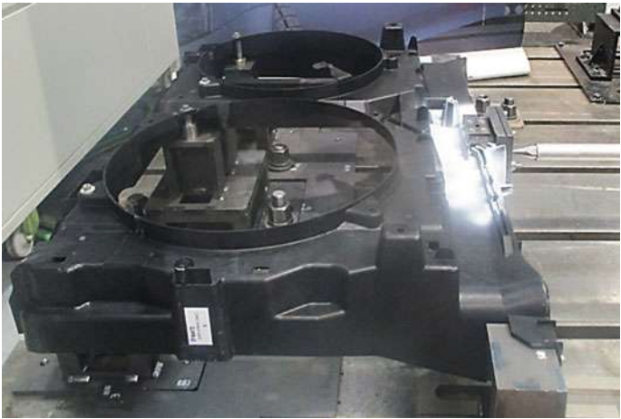
Fig. 12 Front-end carrier validation test
