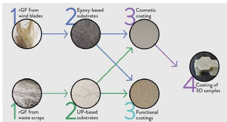
Fig. 1 Workflow of the experimentation from the development of new coatings for rGFRP composites to their preliminary implementation on 3D samples with complex surfaces
