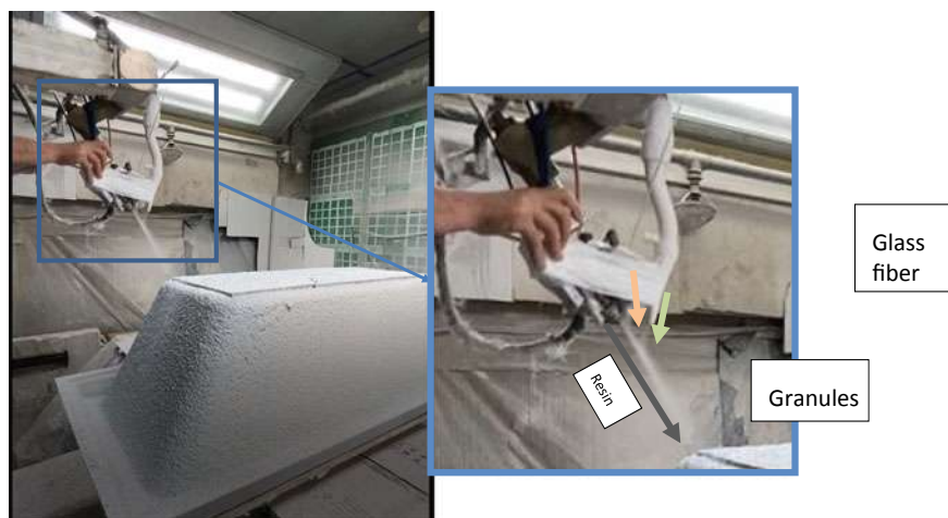
Fig. 7 Production of bath tub demonstrator
