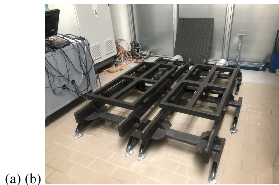
Figure 6: (a) 3D solid model of the uniaxial shaking table. (b) Shaking table frame in laboratory.
