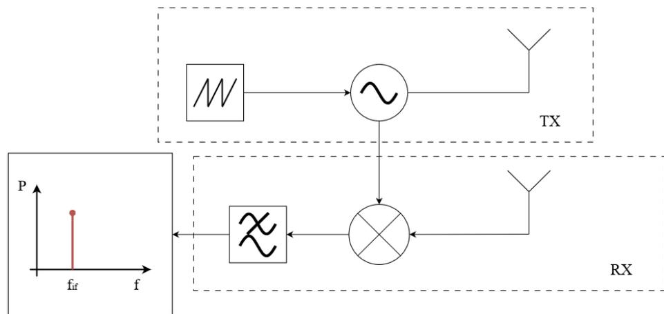
Figure 2. Basic scheme of an FMCW radar.
