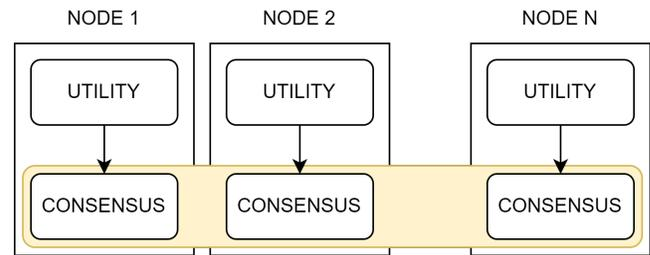
**Figure 1: Each node maintains a utility function to determine its suitability for executing a specific task, and the underlying framework analyzes the outputs from these utility functions to converge on an optimal task allocation.**
