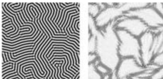
Figure 1: Simulated self-assembly stripe nanostructures (left). The result of applying the unsupervised shapelet-based method to automatically identify grain boundary defects (right).
