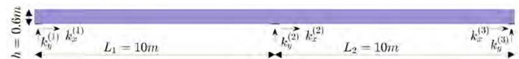
Figure 2. Geometry of the two-span bridge in the longitudinal direction with elastic boundaries.
