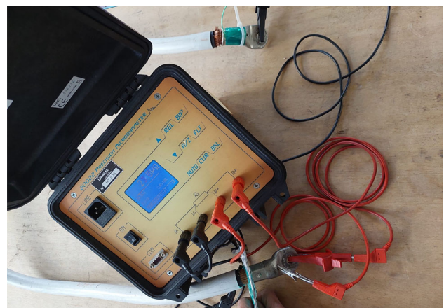
Fig. 7 View of the connection of the microohm-meter to the lug for the direct measurement of R_{\text{crimp}}
