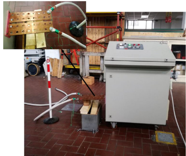
Fig. 9 View of the heating setup with the OS.A.T current generator (right side) supplying, through two copper bars, the cable headed with the two crimped lugs whose R_{\text{crimp}} has to be measured
