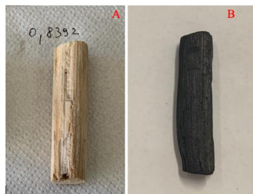
Fig. 3. Example of: A) pre pyrolyzed sample; B) pyrolyzed sample
