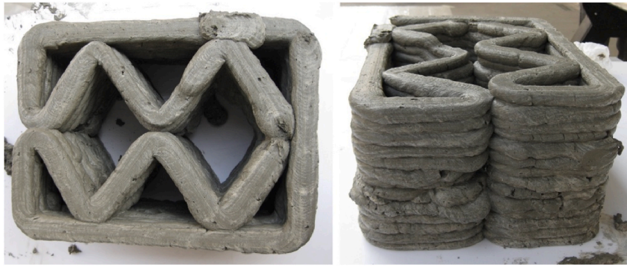
Fig. 13. Representative images of BC.2.1 obtained using 3DCP.
