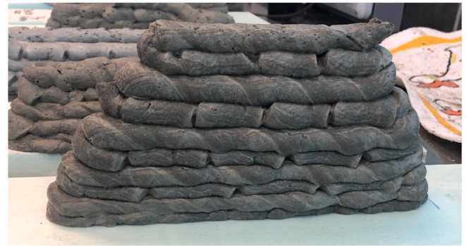
Fig. 3. Result of 2D-printing test conducted on 3DPFC_800.
