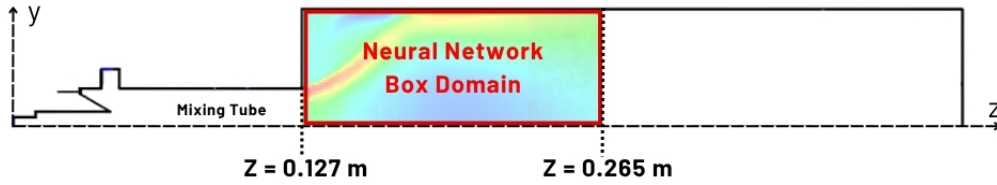
Fig. 8 Computational domain and selected region of interest used for the U-Net-based multi-fidelity correction. The red box identifies the portion of the combustor in which the 2D flow fields are mapped to the corresponding planar fields extracted from the 3D simulation.
