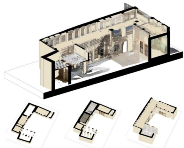
Figure 12 Sectioned views of the BIM model of the Aljazzaf house. The model was generated from the pointcloud. Software employed Autodesk Revit 2016. Images source Authors and Marwa Reyadh Alarayedh.
