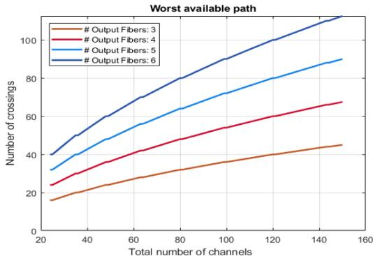
Fig. 8: Number of crossing in the worst path as a function of the number of input channels and number of output fibers (# Output Fibers)
