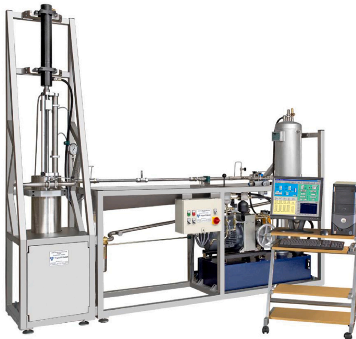
Fig. 13. Overview of the TriFlow Low Flow Liquid Calibrator System TF030 (OM2).
