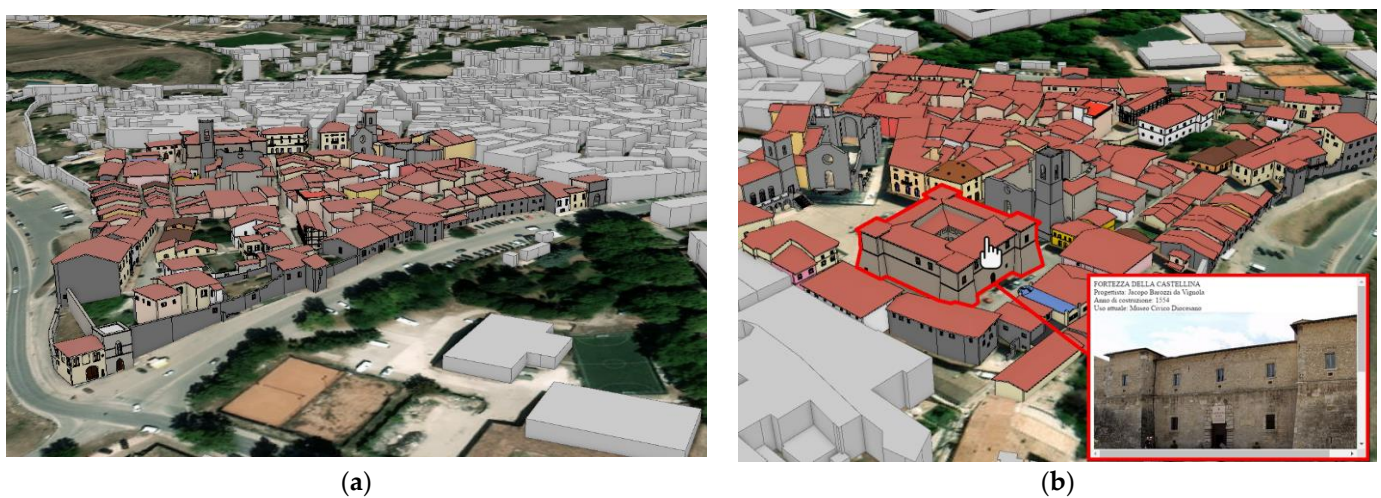
Figure 12. The Urban BIM related to Norcia city centre: the south-west part of the city (a), with a zoomed view on the Castellina 3D model and query in the 3D database (b).
