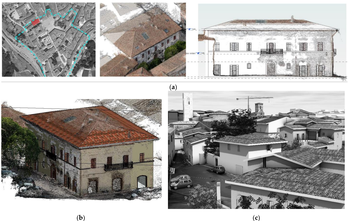
Figure 8. Examples of one sample building definition (building n°2, Via Solferino) based on point clouds with parametric modeling, with eaves, ridges, floors and ground lines (a); corresponding modelling according to LOD 300 (b) in the evacuated residential area; and aerial views of the centre with the other modeled buildings (c).
