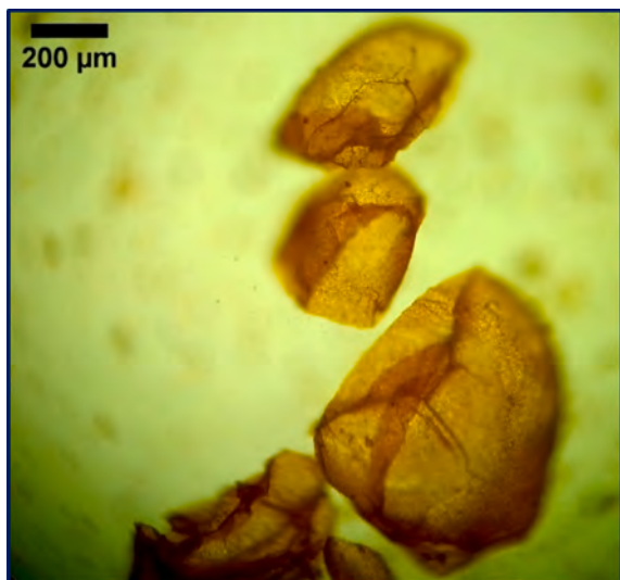
Fig. 17. Sample Emu W/O 16 left in air on a glass slide for 30 min. The resulting deflated structure demonstrates that the particles are strongly adsorbed at the interface.
