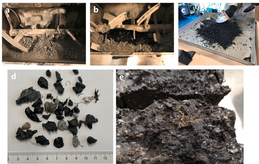
Fig. 4. Preparation of asphalt mixture with PE waste plastic a) Hot aggregates and PE waste plastic; b) Addition of binder; c) Final mixture; d) PE waste batch 3; e) Partially melted plastic in the asphalt mixture (Courtesy Lab 6 and Lab 7).
