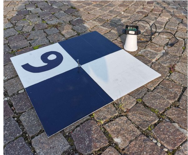
Figure 2. Example of target and Pozyx UWB anchor.
