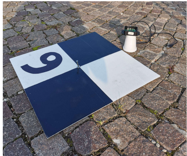
Figure 2. Example of target and Pozyx UWB anchor.
