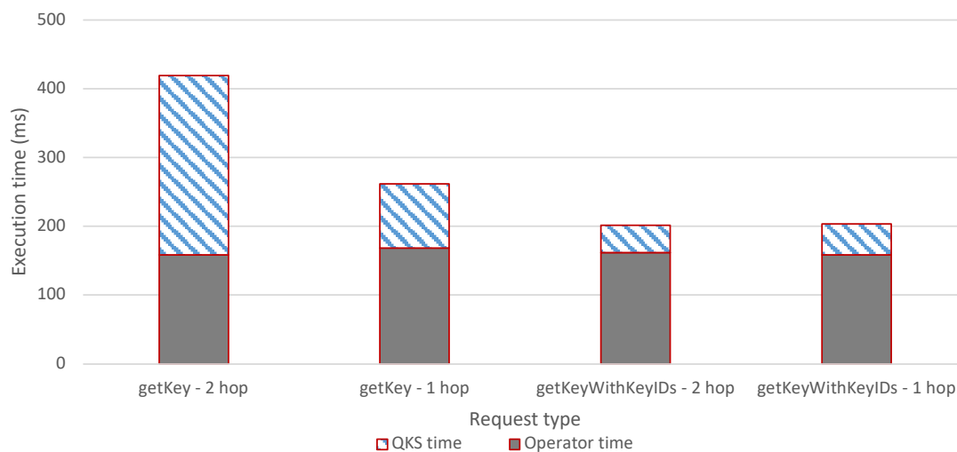
Fig. 4.10 Execution time of the getKey and getKeyWithId functions for Point-to-Point and Multi-hop exchanges.
