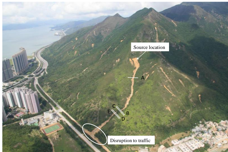
Figure 1: Picture of the Yu Tung debris flow. The five sections indicate chainages (CH) where velocity estimates are available: A: CH100; B: CH413; C: CH439; D: CH462; E: CH477.
