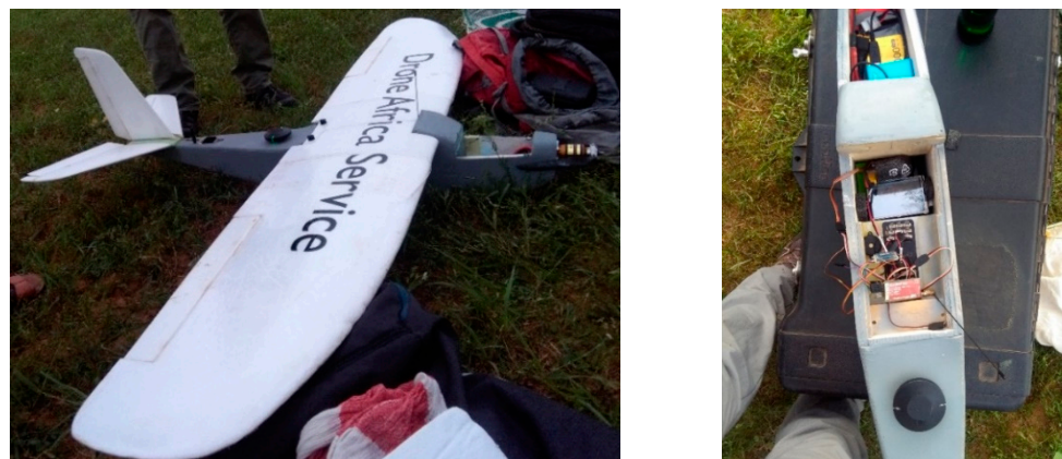
Figure 3. Left: UAS system built by Drone Africa Service. Right: Detail of the UAS body. It is visible that the Raspberry Pi sensor is mounted on the UAS system; 3.5-inch screen and the GPS receiver.
