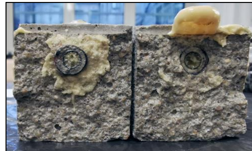
Fig. 1. Cross-section of a PUC specimen after failure showcasing the ruptured resin capsule and the the spilled resin.
