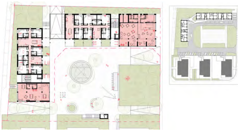
Fig. 2. Preliminary hypothesis of the ground floor plan for the feasibility study, with communal areas highlighted in pink (left), and ground floor plan of the building before intervention, 2023 (Drawings reworked by the authors of the paper).
