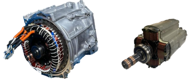
Fig. 9. 100 kW EESM sample for the validation current-to-flux data.
