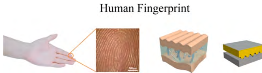
Fig. 27. Example of electronic application of mechanical interlocking structures. Flexible piezoresistive sensor inspired by the structure of human fingerprints, incorporating micro-features between soft-rigid polymers to enhance sensing performance and mechanical stability. Adapted with permission from [137]. Copyright 2024 American Chemical Society.
