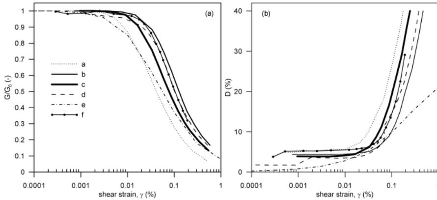
Figure 5. Dependence of shear modulus (a) and damping ratio (b) on strain level.
