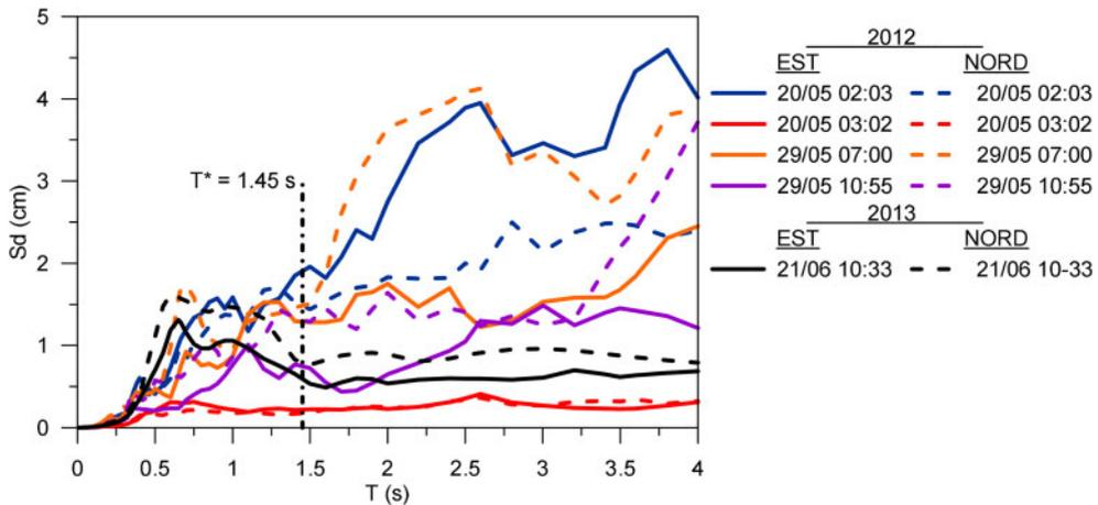
Figure 10. Displacement spectra of May 2012 and June 2013 seismic events.
