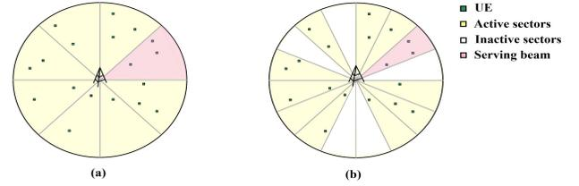
Figure 1. Pictorial representation of a 2-D single cell with 20 independent and uniformly distributed UEs, served by a single analog beam when the cell sectorization scheme is (a)  $S = 8$  sectors, and (b)  $S = 16$  sectors.
