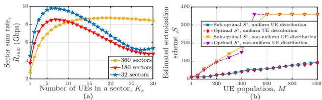
Figure 6. (a) Plot of sum rate per sector versus number of UEs in the sector for three different sectorization schemes. (b) Comparison of optimal  $S^*$  obtained through exhaustive search method and sub-optimal  $\hat{S}^*$  obtained using reduced complexity search method for uniform and non-uniform UE distribution.
