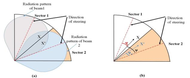
Figure 2. (a) Pictorial representation of true position  $\mathbf{X}$  and estimated position  $\mathbf{X}'$  of a UE along with the actual beam coverage region considering practical radiation pattern. (b) Demonstration of EAOA of the UE;  $\Psi$  is the true EAOA and  $\Psi_e$  is the estimated EAOA with respect to sector 2, whereas  $\Psi_a$  is the true EAOA of UE with respect to sector 1.
