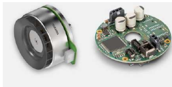
Figure 21. Chosen motor (left) and the inverter (right).
