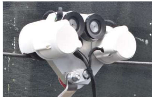
Figure 24. Trolley traction structure with 3D-printed cover.
