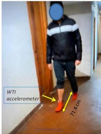
Figure 3 The Cagliari's testing subject is shown with the WTI accelerometer fixed to the outside of the right ankle, performed without shoes a 10 strides walking task in which each stride was of 71.4 cm and lasted 1 second.
