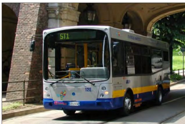
Figure 18. The “Linea Star” bus line 1 in Turin, the EPT-Cacciamali “Elfo” electric minibus (2003–2022).
