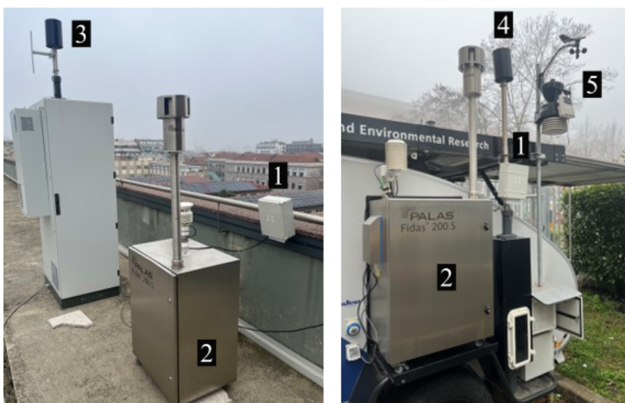
Fig. 2 Positioning of ENEA MONICA microsenors and reference instruments for calibration at DIATI – Politecnico di Torino. Left: CC-Green Roof. Right: CC-TrAIRer Lab. 1 – ENEA MONICA™ microsenors, 2 – Palas Fidas 200S optical sensor for PM measurement, 3 – Sampling head for ENVEA AC32e analyzer for NO 2 measurements, 4 – Sampling head for Serinus 40 analyzer for NO 2 measurements, 5 – Davis Vantage Pro 2 weather station.
