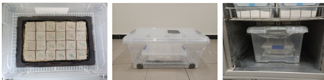
Fig.4-11 Experimental setup and procedure for water retention curve measurement via the semi-permeable membrane method
