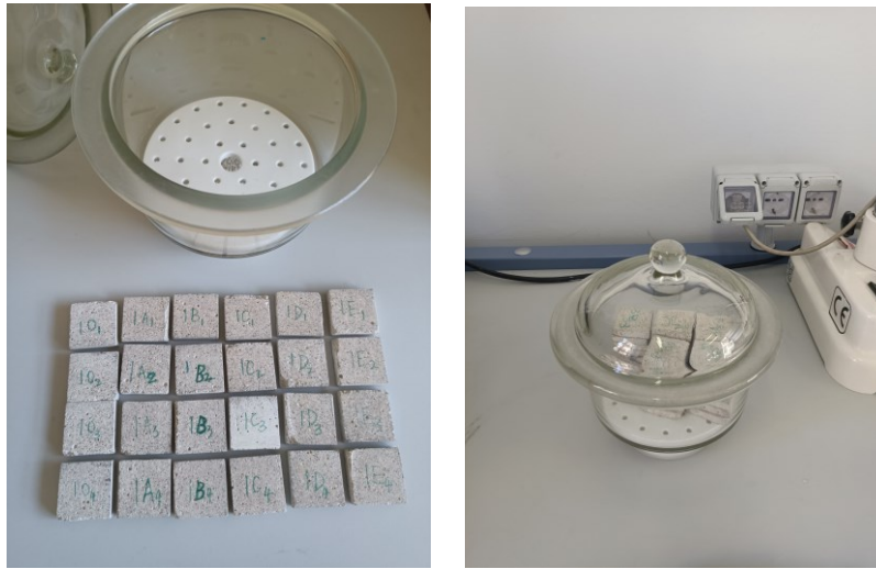
Fig. 5-5 Glass container for sealed specimen weighing
