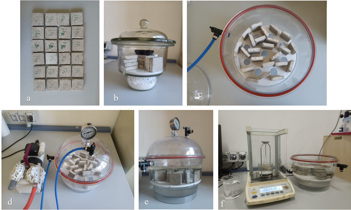
Fig. 4-6 Vacuum saturation experimental setup and procedure
