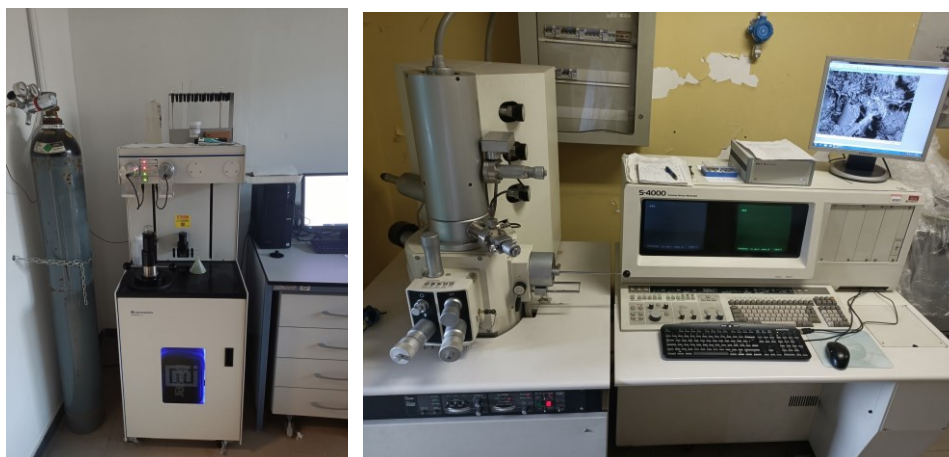
a) MIP (Autopore V) mercury intrusion porosimeter b) SEM (Hitachi S4000) scanning electron microscope
