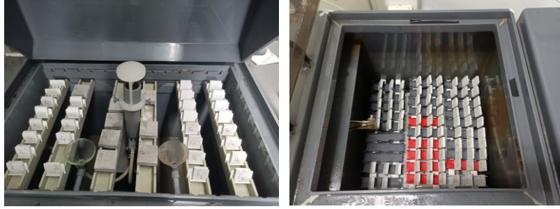
Fig. 2-6 Placement of cement mortar specimens inside the salt spray chamber
