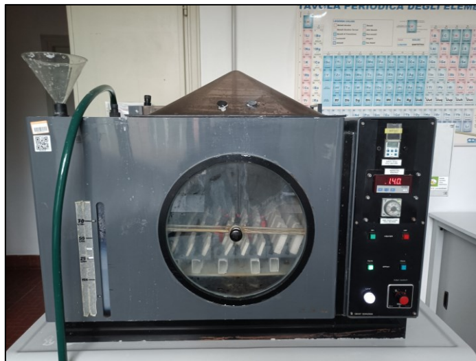
Fig. 2-2 CEAST 5050 salt spray test chamber
