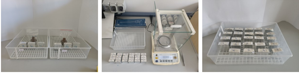
Fig. 4-9 Capillary absorption experimental setup and procedure
