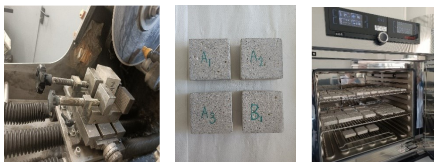
a) CNC cutting b) Cleaning and labeling c) Constant-temperature drying
