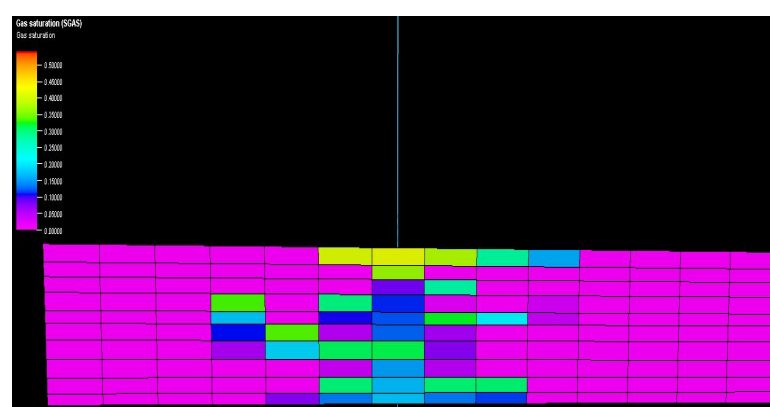
Figure 11. Vertical cross section of reservoirs showing gas saturation in heterogenous model.
