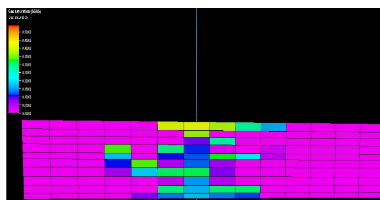
Figure 11. Vertical cross section of reservoirs showing gas saturation in heterogeneous model.
