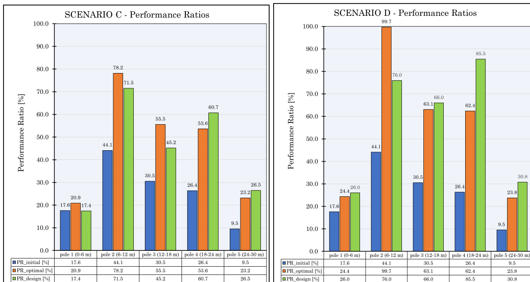
Fig. 5.15 Scenarios C, D. In blue, orange, and green, the average PRs, respectively, at the initial condition, after optimization, and the design solution.
